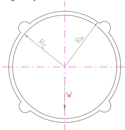
Fig. 2 Cylindrical four-groove bearing
