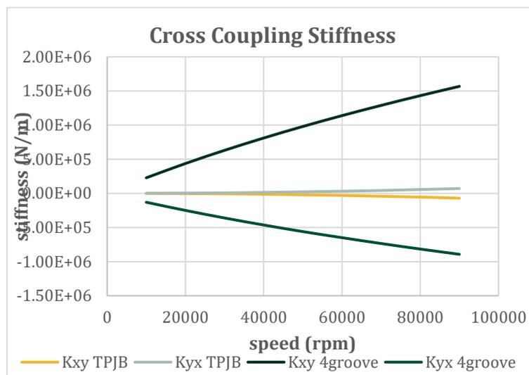
Fig. 4 Cross-coupling stiffness terms of cylindrical four-groove bearing and TPJB
